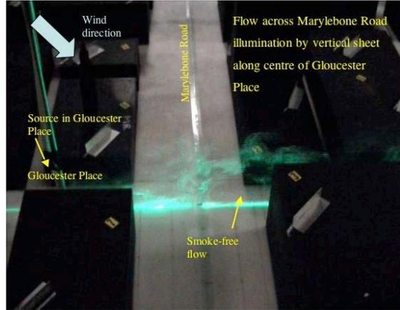
The smoke source is as before and a vertical light sheet is directed along the centre of Gloucester Place, from the south. Plume ‘lift-off”, illustrated here at about the centre of Marylebone Road, is frequently observed in the video recording from which these stills have been taken. There is a continuous flow of smoke into Gloucester Place north.
