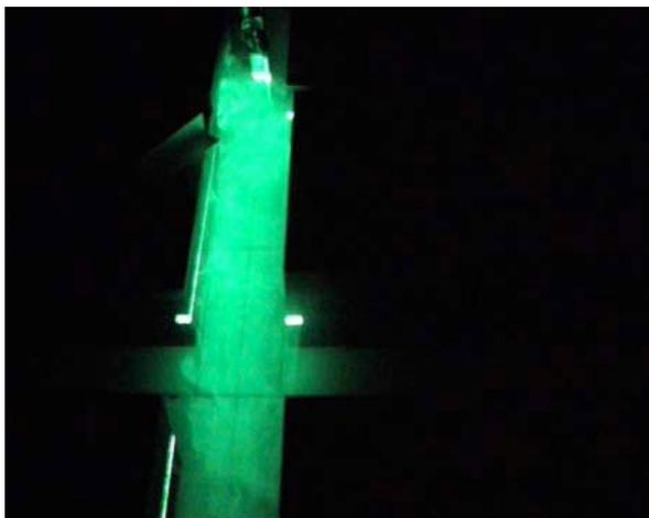
This “branching” situation is not at all common. Much more frequent is a sequence in which a fraction of the flux in the smoke plume crosses the intersection and becomes detached from the main plume (at least at this height). The sequence on the next page illustrates this. However, the most common behaviour is that shown in the larger image above.
