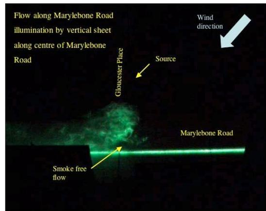
Taken together, the three sets of images show smoke flow from Gloucester Place South into both Marylebone Road and Gloucester Place North, the exchange being associated with significant three dimensionality in the flow at the intersection.
