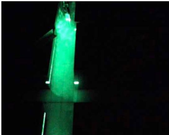
The sequence runs from left to right, top to bottom. A small smoke 'cloud' becomes detached from the main plume and continues along York Street. There is however vertical motion perpendicular to the plane of the light sheet, so the term 'detached' should not be taken too literally. For example, other observations, not included here, show some smoke escaping from the York Street canyon and travelling above roof level.
