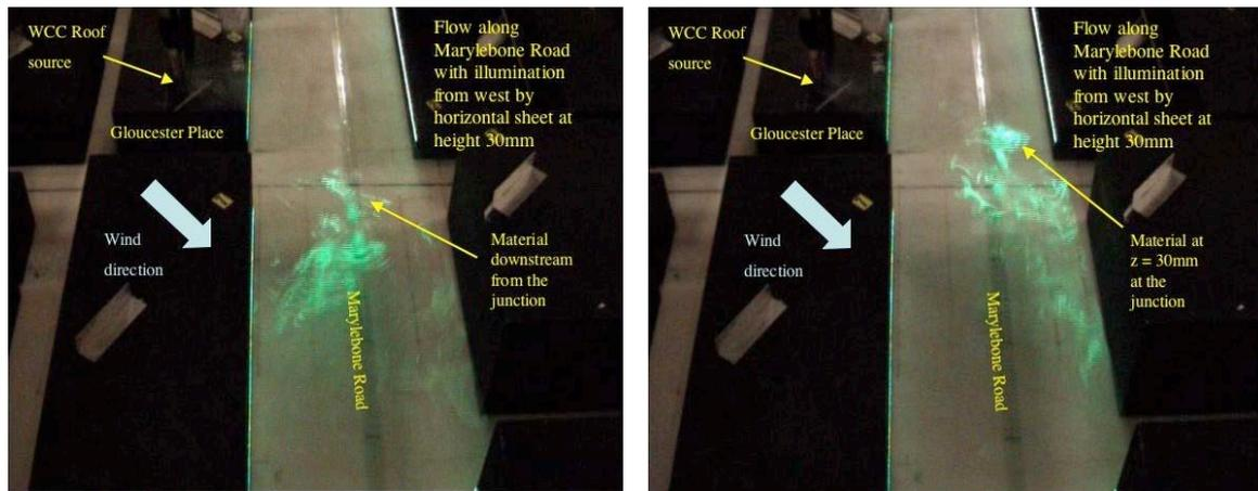
The roof-top source is located half-way along the Gloucester Place side of the building, half-way between the roof edge and the central tower. The light sheet is directed along Marylebone Road at a height of 30mm. At this level the distribution of smoke in the region shown above is highly variable. Overall, it is most likely to be seen in the central or northern part of the Road and not in the large recirculation region on the south side.
