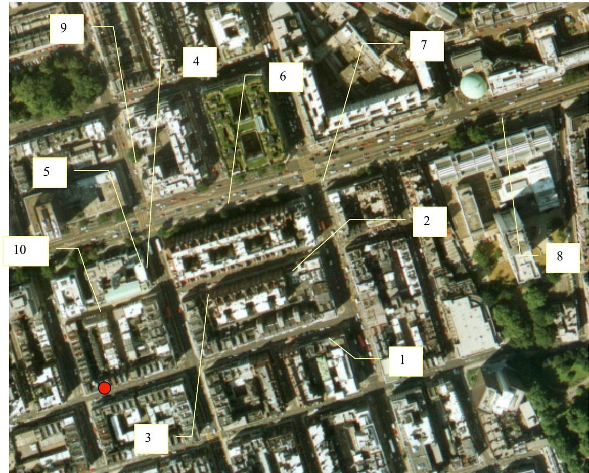
Figure 1: Area map of the tracer field study (Marylebone area) depicting source-receptor positions; source indicated by red the spot, and receptors are numbered and indicated by the yellow lines.
